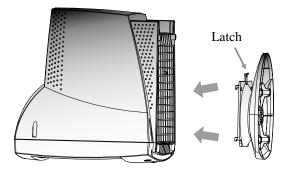
If you want to remove the tilt/swivel stand on the monitor, press the latch and pull the tilt/swivel stand toward the back of the monitor. Lift the stand to separate.
